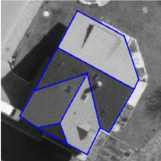
Figure 6: Result of automatic roof reconstruction (source: [7]).
